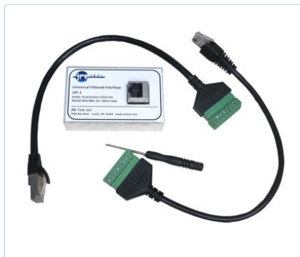
Shown with the two supplied pendant cables and terminal blocks
