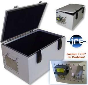
Universal I/O plate allows almost any device to be interfaced inside the enclosure, and internal electromagnetic absorbing material reduces RF reflections and hot-spots. Unit shown with populated I/O plate for illustration.
