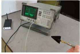
the 20 dB minimum path loss of 2.45 GHz at a meter distant and you end up with an isolation figure of 100 to 110 dB. This is a fast, easy reliable test of the shielding. Its not a bad idea to perform this test periodically to ensure your enclosure is operating correctly, especially after reconfiguring or shipping.
